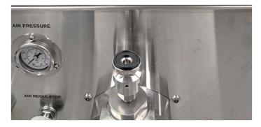
Place the sample holder on top and hold it in place with the metal clamp. This only needs to be finger tight.
