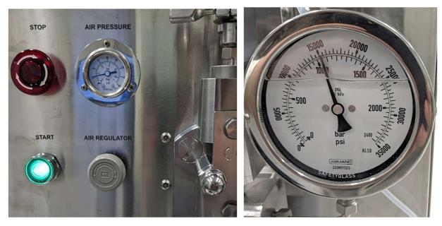
Turn the main switch on, in the back. The red STOP button should light up.
