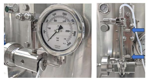
OPTIONAL: Connect the cooling tubes from the water cooler to the extruder (blue arrows).
