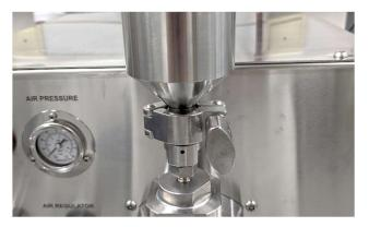
Place the pressure gauge on the side, as shown below, tightening it with a 17 mm wrench. No need to overtighten. Place the extruder in front, as shown below, tightening it with a 17 mm wrench. No need to overtighten.
