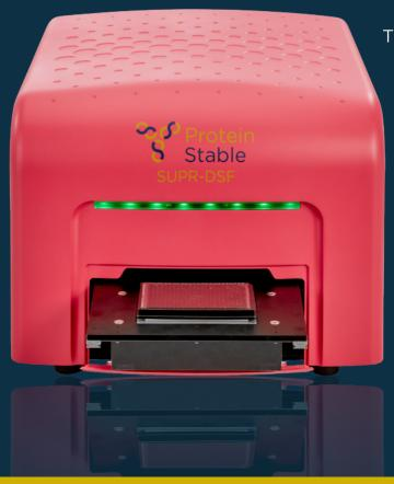
The SUPR-DSF by Protein Stable delivers level differential next scanning fluorimetry by simplifying sample preparation and analysis of protein stability into a single microplate. Utilising precision optical components to deliver the highest sensitivity, intrinsic fluorescence of proteins and full spectrum detection, both thermal ramping and isothermal chemical denaturation experiments can be easily run in 384-well microplates.
